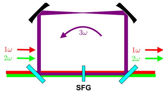
**FIGURE 1.** RING principle [1] adapted to laser ion stripping. Fundamental frequency ( $\omega$ ) and the second harmonic ( $2\omega$ ) laser pulses are injected into the cavity and rejected from the cavity using a pair of dichroic mirrors. A sum-frequency generation (SFG) crystal generates the third harmonic pulse ( $3\omega$ ), which is recirculated in the cavity with all mirrors designed to be highly reflective for the third harmonic.
