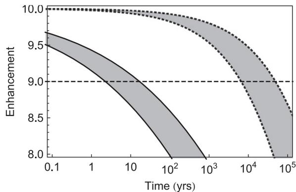
**FIGURE 3.** Expected variation of the enhancement factor for a RING cavity with pre-irradiation cavity loss of 10, for linear model (dotted) and quadratic model (solid). Shaded is the range of the expected enhancement, reflecting the uncertainty associated with mixed irradiation by fast neutrons and gamma-rays. The dashed line indicates the enhancement factor drop of 10% from its pre-irradiation value.
